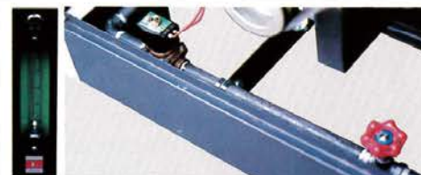
Automatic interlocking dumper for intake/exhaust For controlling drop/rise in the temperature.
